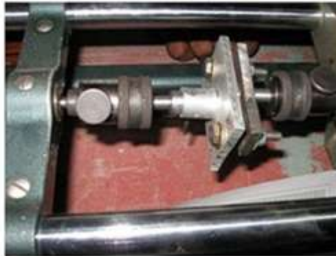
Fig. 10 Tensile test conducted using a tensometer
